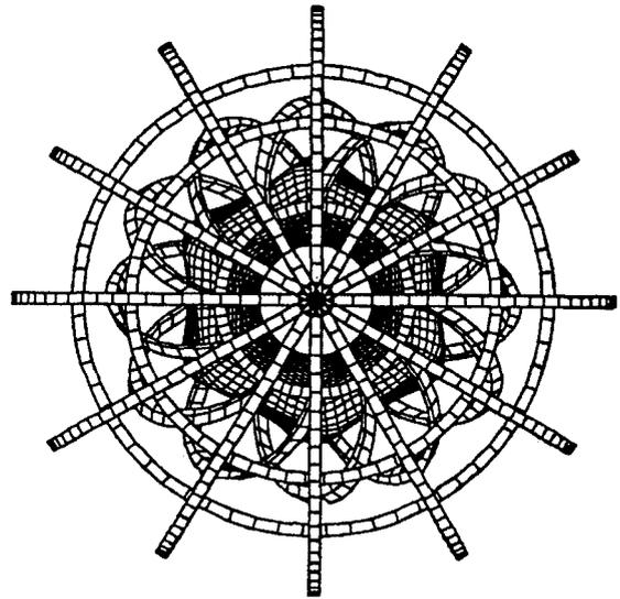
FIG. 4. Top view on the configuration with the classical stellarator type OSW.
