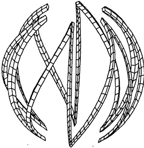
FIG. 6. Torsatron type OSW.
