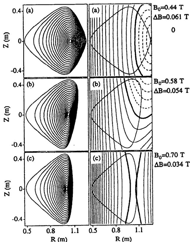
FIG. 2. Left side, closed vacuum flux surfaces produced by the classical stellarator type OSW: (a)  $\varphi = 0$ , (b)  $\varphi = \pi/(2N)$  and (c)  $\varphi = \pi/N$ . Right side,  $|B|$  distributions in the corresponding cross-sections, where  $B_0$  corresponds to the bold contour lines and  $\Delta B$  is the difference between neighbouring contours.
