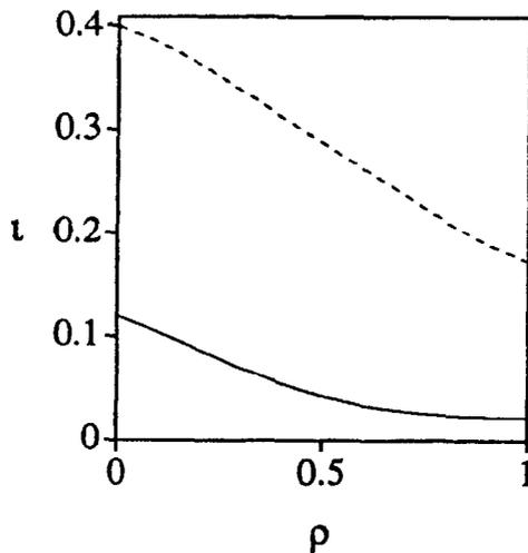
FIG. 10. Total rotational transform for the currentless equilibrium of Fig. 8 (solid curve), and for the current carrying equilibrium of Fig. 9 (dashed curve).
