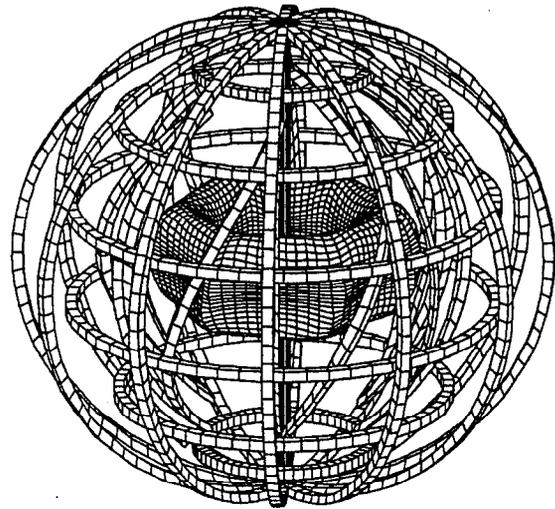
FIG. 7. Side view on the configuration with the torsatron type OSW.
