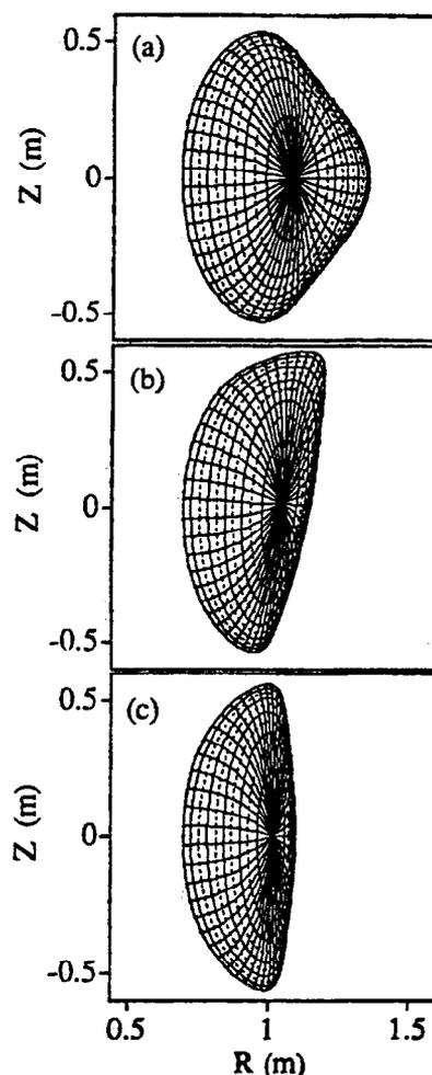
FIG. 9. MHD equilibrium with  $I_p = 120\text{ kA}$  and  $\langle\beta\rangle \approx 4\%$ .
