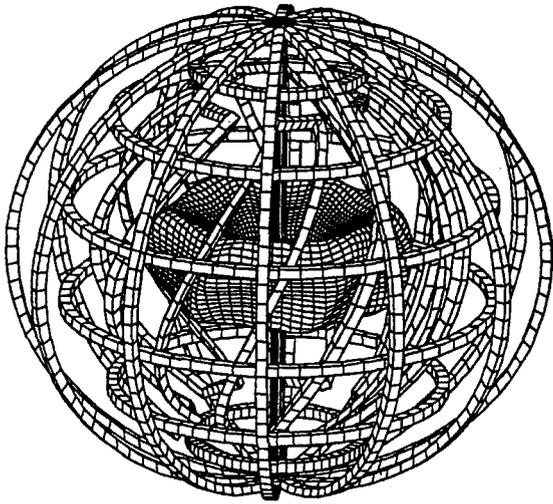
FIG. 3. Side view on the configuration with the classical stellarator type OSW.
