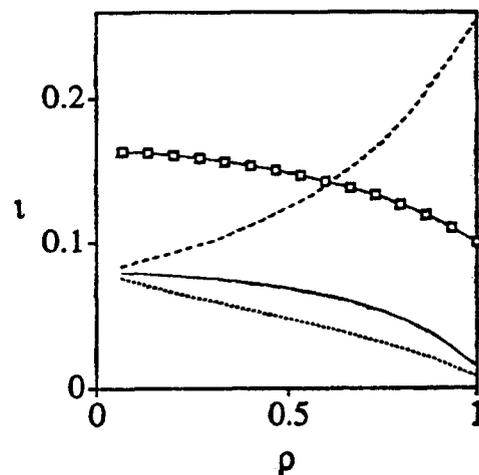
FIG. 5. Radial profile of the total rotational transform (solid curve) and its outboard (dashed) and inboard (dotted) components. The curve with squares corresponds to the increased current,  $I_{OSW}$ .
