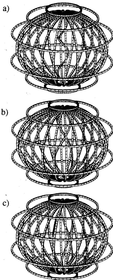
Fig. 1. The coil systems of the SHS (a), DHS (b), and THS (c).
