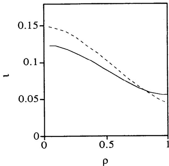
Fig. 4. Radial dependence of the rotational transform for the SHS without PF rings (solid curve) and with PF rings (dashed curve).
