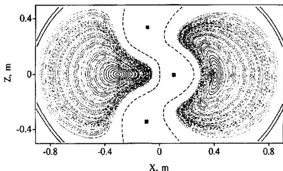
Fig. 3. Poincaré puncture plots for closed vacuum flux surfaces in the  $X$ - $Z$  cross-section of a SHS without PF rings. The dashed curves demonstrate the geometry of opened field lines around the helical post. Cross-sections of the coils are shown as well.
