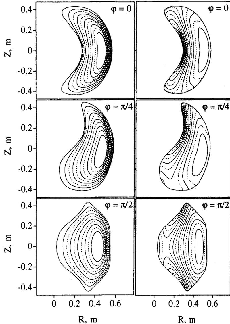
Fig. 7. High  $\beta$  ( $\beta_0 = 86\%$ ,  $\beta = 20\%$ ) MHD equilibrium in the DHS with the self-consistent bootstrap current. Flux surfaces (left column) and contours of  $|B|$  (right column) are shown.
