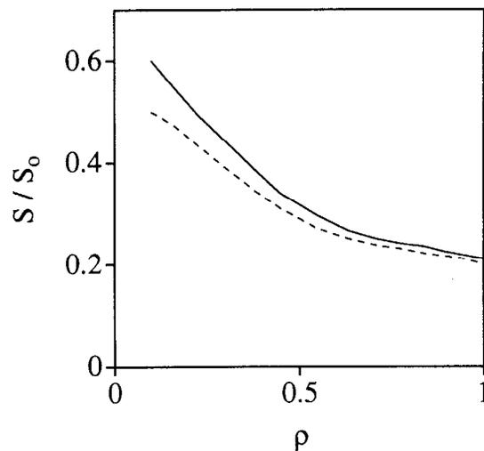
Fig. 5. Radial dependence of  $S/S_0$  for the SHS without PF rings (solid curve) and with PF rings (dashed curve).
