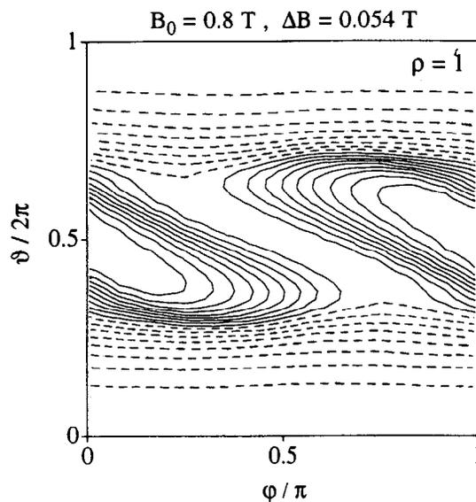
Fig. 6.  $|B|$  distribution on the last closed vacuum flux surface of the DHS. Solid contours are for  $B \geq B_0$ , dashed for  $B < B_0$ ,  $\Delta B$  is the difference between adjacent contours.
